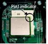
2. Locate Pin 1 in the socket and look for a (golden) cut edge on the CPU upper corner. Then insert the CPU into the socket.
